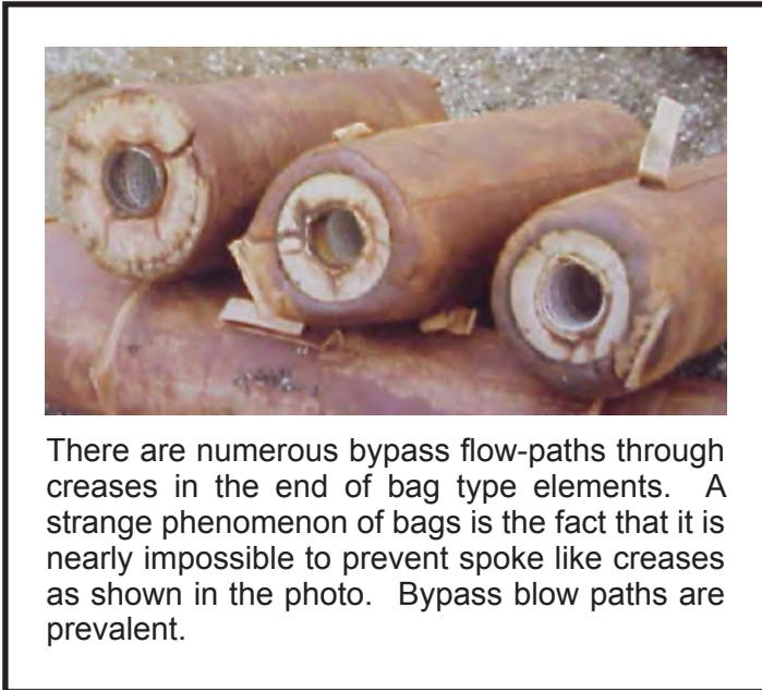
There are numerous bypass flow-paths through creases in the end of bag type elements. A strange phenomenon of bags is the fact that it is nearly impossible to prevent spoke like creases as shown in the photo. Bypass flow paths are prevalent.
